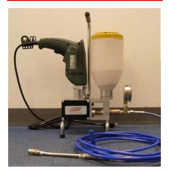
Tam Drill Pump is a light weight and handy electrically operated pump used for high pressure chemical grouting. It is a simple to use injection pump especially designed for the injection of single shot polyurethane grouts or epoxy resins. It is the perfect machine for daily use and suitable for performing both commercial work and residential injection, with its compact design it is ideal for use in confined areas.
